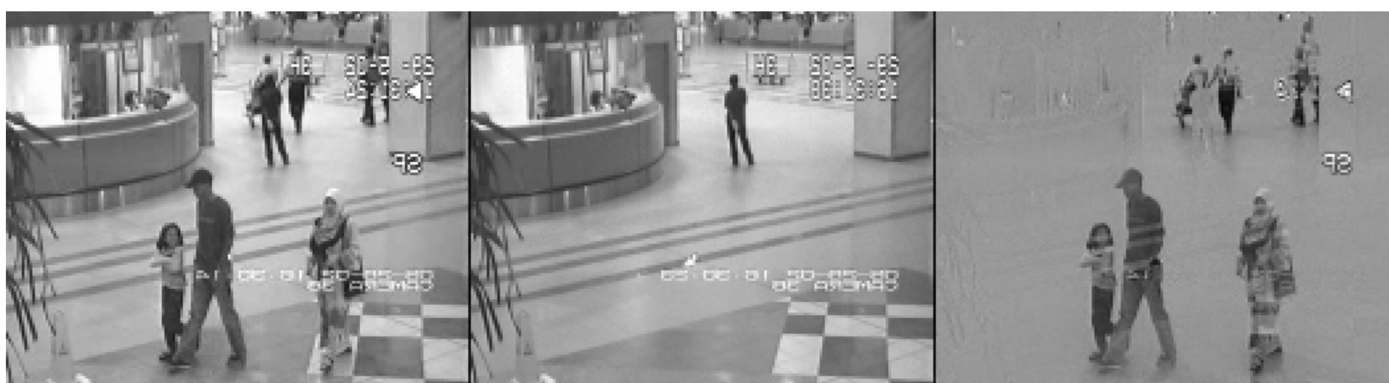
Fig 2. BEAR for surveillance camera data. (Left) Input video ( Y ) (Middle) L , (Right) S
